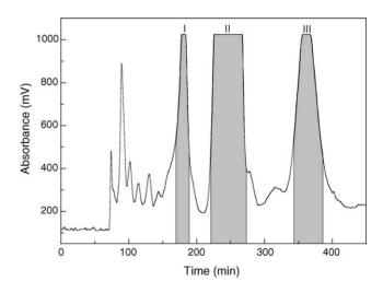
Fig. 3. HSCCC chromatogram of crude extract from *Epimedium koreamum* Nakai. Two-phase solvent system: chloroform–methanol–water (4:3.5:2, v/v); mobile phase: the lower phase; flow-rate:  $2.0 \text{ ml min}^{-1}$ ; revolution speed: 900 rpm; detection wavelength: 254 nm; sample size: 200 mg of crude sample dissolved in 4 ml of the upper phase; separation temperature:  $25 \,^{\circ}$ C; retention percentage of the stationary phase: 50%.
