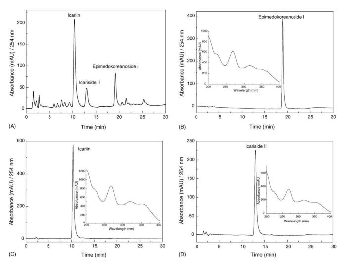
Fig. 2. HPLC chromatogram of crude extract from *Epimedium koreanum* Nakai and HSCCC peak fractions. Conditions: column: reversed phase YWG  $C_{18}$  column (200 mm × 4.6 mm i.d., 10 µm); mobile phase: acetonitrile and water in gradient mode (acetonitrile: 0–12 min, 28%; 12–20 min, 28–35%; 20–30 min, 35%); flow-rate: 1.0 ml min<sup>-1</sup>; detection wavelength: 254 nm. (A) Crude extract from *Epimedium koreanum* Nakai; (B–D) HSCCC peak fractions I–III in Fig. 3.
